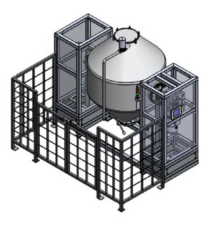
The automatic stop positions are: loading, unloading and sampling. Before stopping in one of the above three positions, it performs a cycle that will slow down the mixer so that it can be accurately positioned and brought to a stop.
