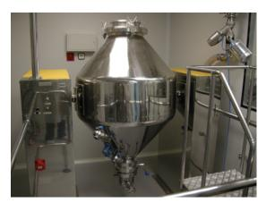
Double cone blender with an automatic loading/discharge system
